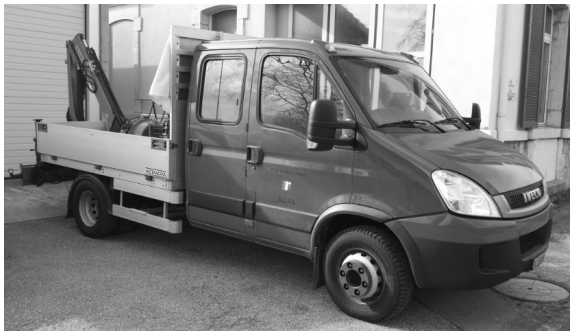
Illustration 3. Van for verification of medium size weighing instruments, equipped with a crane, 2-4 racks containing 20 kg weights, set of 500 kg weights, sets of additional weights & diverse accessories
