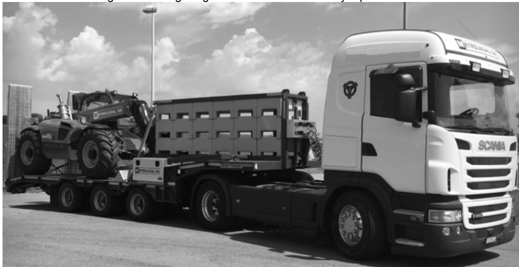
Illustration 4. Truck for weighweight bridge verification, total weight 40 t, equipped with a set 500 kg and 1000 kg weights that can be handled by a pallet truck
