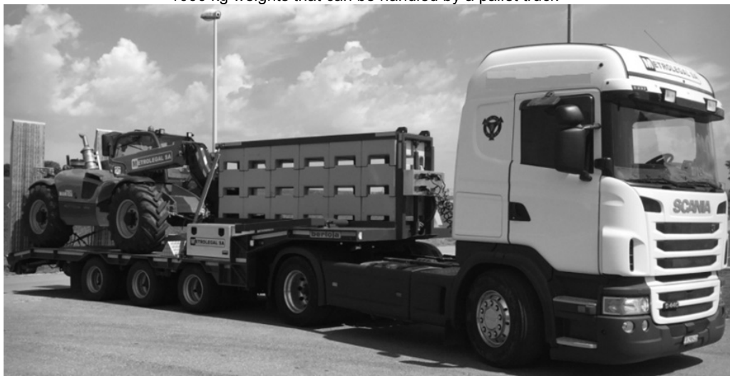
Illustration 4. Truck for weight bridge verification, total weight 40 t, equipped with a set 500 kg and 1000 kg weights that can be handled by a pallet truck
